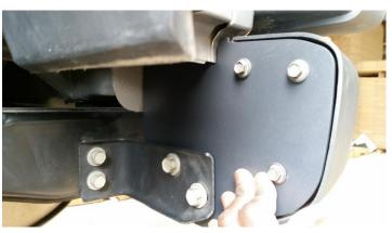
Align the position of your end cap to the bumper and tighten the three 6 MM bolts. Adjust the bumper bracket on the chassis and tighten the two bolts you left loose in step (B). Finally tighten the remaining two bumper bracket bolts.
