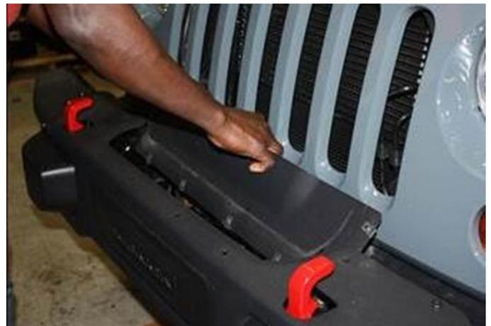
**2- Remove U-nuts from the Bumper and the Cover Plate**
