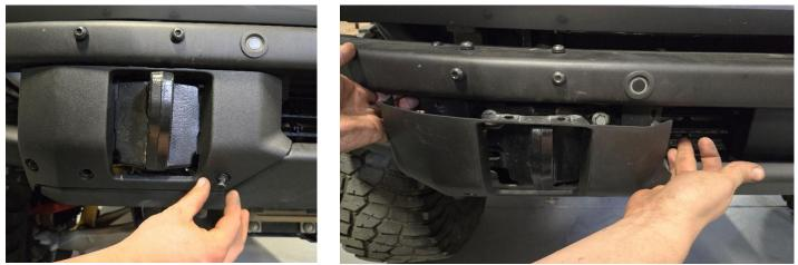
**D. Remove the bumper** by unbolting the 6 bolts (3 on each side) that hold the OEM bumper in place using a 15mm socket. Save all the factory bolts for reinstallation later.
