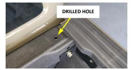
Place Rear Side Tube on the vehicle as shown, align tube flanges to corners of the bed and Corner Brackets to locate and temporally bolt down using M8 Button Socket Bolts.
