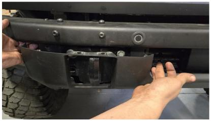
**D. Remove the bumper** by unbolting the 6 bolts (3 on each side) that hold the OEM bumper in place using a 15mm socket. Save all the factory bolts for reinstallation later.
