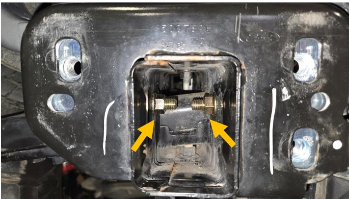
G. Reinstall your bumper and skid plate using your original bolts removed in step A and D.
