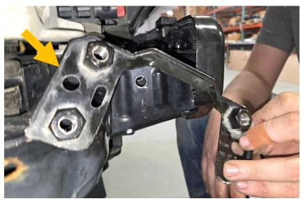
**F. Install the Maximus-3 brackets** as shown below using M12 bolt, serrated nuts and washers supplied. Note outer and inner brackets, driver and passenger side brackets, and their orientation. The single nut bracket goes on the outside of frame.
