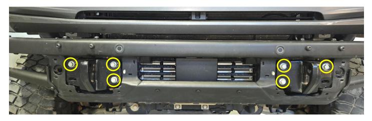
**E. Remove the mounting nut plate** from behind the frame horns, one on each side. You will not need the brackets again for this installation.
